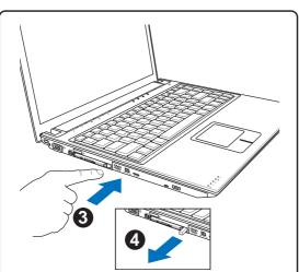
2. Press the extended button again to eject the PC Card. Carefully pull the ejected PC card out of the socket.
